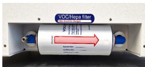
Figure 12.3 Correctly installed VOC/HEPA filter
