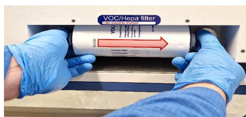
Figure 12.2 VOC/HEPA filter insertion and removal procedure
